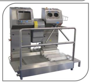
a second photocell unlocks the turn-style of  $\frac{1}{3}$  turnover and switches on the brushes.
