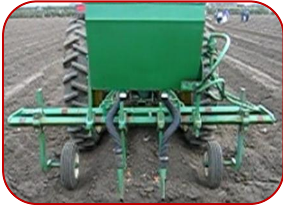
Figure 6.4: 'Clampco' precision applicator provides free flow of Multicote™ Agri
